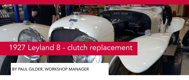
When your average modern car needs a new clutch, it's half a day at the local garage and a new clutch kit from the manufacturer. Not so easy with older cars! The Leyland 8 came into the workshop as it was time for a full inspection. On this particular car the starter motor drives through the gearbox and clutch to the engine, so signs of a slipping clutch show during the starting procedure as well as while driving. And the signs were there.
